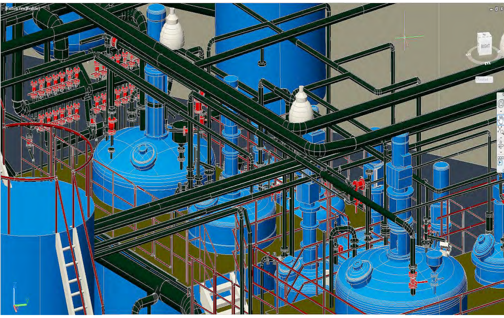
‘Digital Twin’ of production: “All Reactors and mixers modelled with all details like sensors, valves, flanges, drains...”
